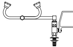
**W-0927-00 Panel Mounted Eye Wash Fixture** Consists of stainless steel bowl, two Gentle Spray outlet heads, a "PUSH TO OPERATE" ball valve and mounting bracket. 1/2" I.P.S. female thread inlet and 1 1/4" I.P.S. female thread outlet.
